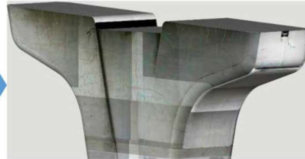
Display the distribution of cracks pasted on a 3D diagram
